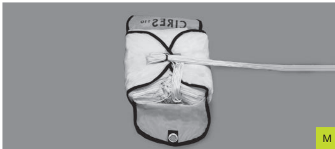
Stow the lower suspension lines in a “figure 8” pattern, securing each loop end with a rubber band twisted in a figure “8”. Keep the suspension lines with the same length and equal tension. (Image N)
