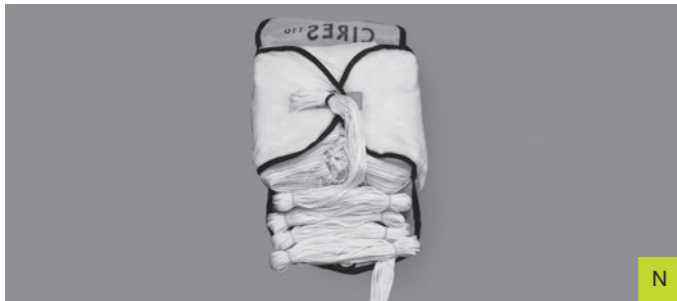
Stow the lower suspension lines in a “figure 8” pattern, securing each loop end with a rubber band twisted in a figure “8”. Keep the suspension lines with the same length and equal tension. (Image N)
